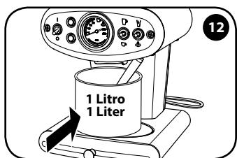
Refit a container of at least 1 litre capacity under the coffee dispensing spout.
